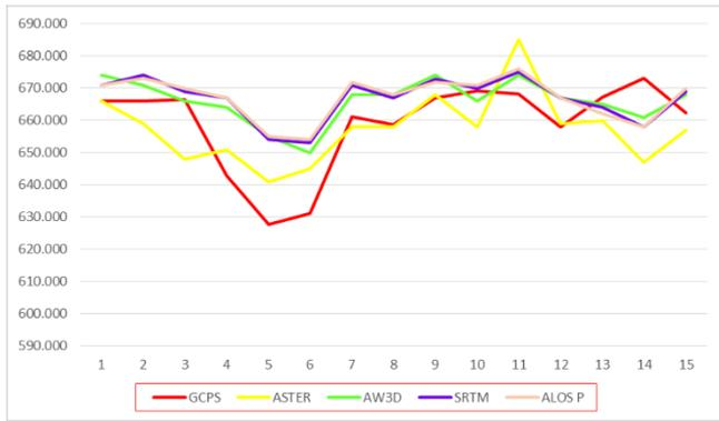
**Figure 2.** Scattered plot for spot height of the various DEMs for plain terrain
