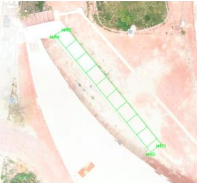
Figure 5. Stair steps that can only be distinguished from 50 meters altitude
