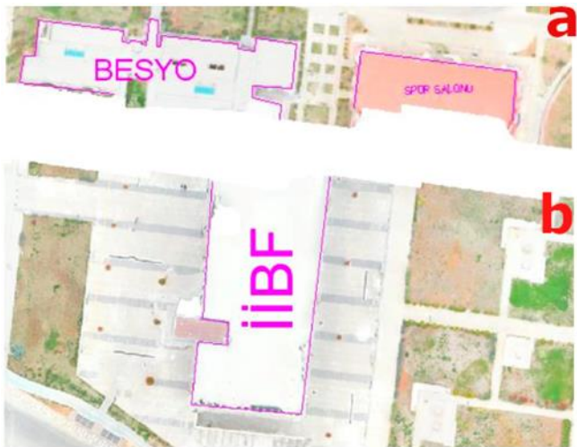
Figure 6. (a) missing building corners at 50 meters height, (b) building visible from 120 meters
