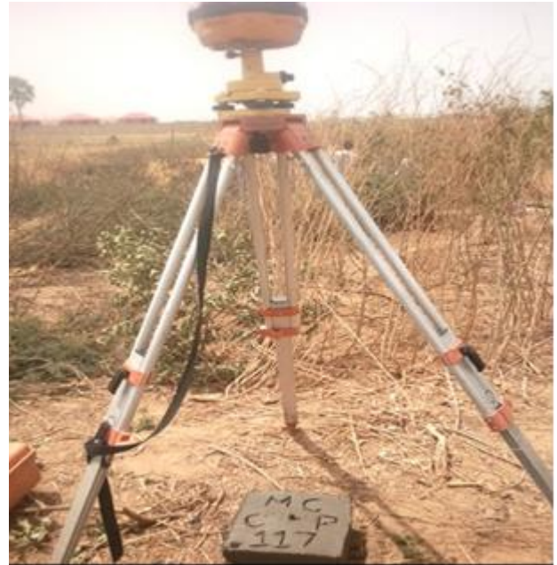
Figure 3. GNSS Static Mode Observation in Progress
