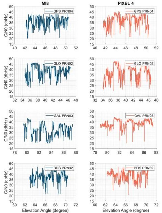
**Figure 2.** C/N0 values of specific GNSS satellites for Xiaomi Mi 8 and Google Pixel 4 smartphones
