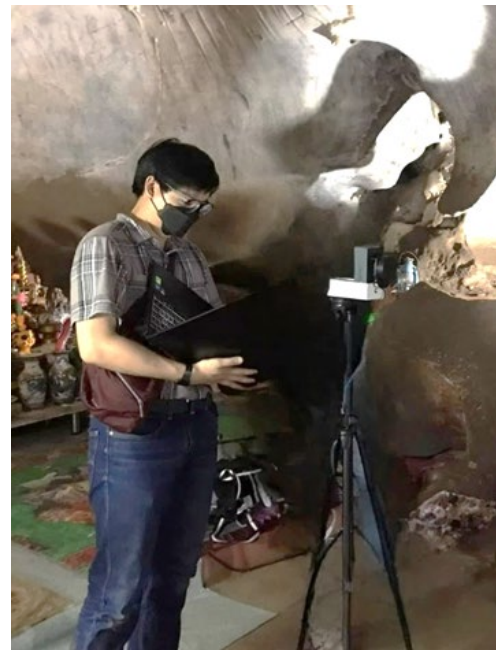
Figure 3. Cave profile scanning in the Muang-On show cave, Chiang Mai, Thailand. The equipment used exhibits the modified 2D LiDAR carefully attached to a camera tripod connected to a laptop. The LiDAR sensor rotates vertically to measure the distance between cave walls, floors, and roofs to create a single cave profile.
