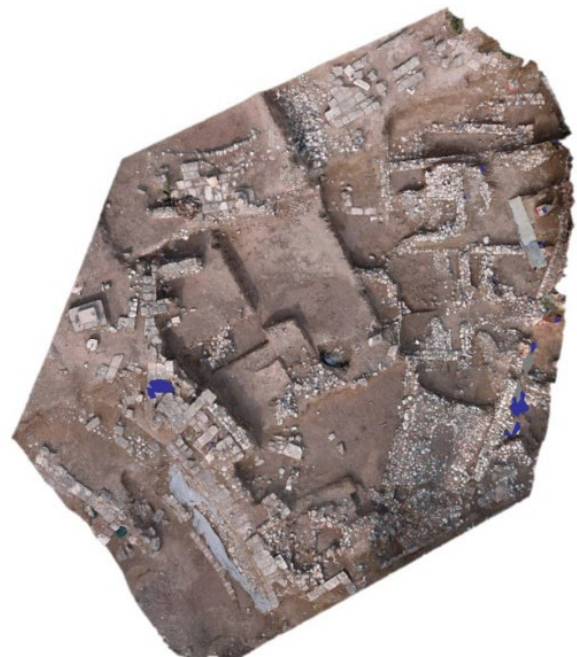
Figure 4. Point cloud obtained in Agisoft Metashape software using UAV images.
