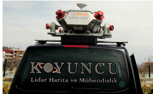
Figure 2. High Speed, High Performance & Dual Browser Mobile Mapping System RIEGL VMX-450 (courtesy Koyuncu Lidar)
