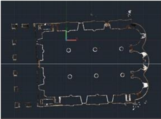
Figure 4. Point cloud slice plan section and drawing
