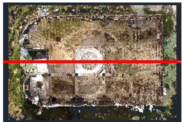
Figure 5. Section line over the 3D point cloud
