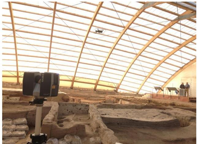
**Figure 8.** Terrestrial Laser Scanning with FARO Focus3D 120
