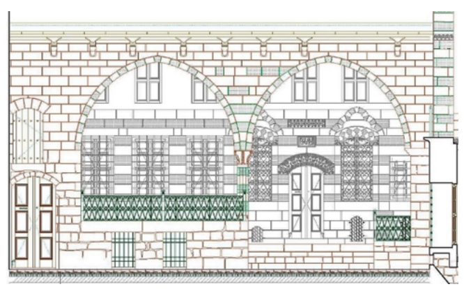
Figure 17. Analytical survey of the east façade of the building facing the courtyard
