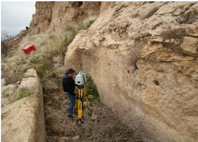
Figure 2. Sample photograph of documenting the rocks of the south façade cliff section with a laser scanner (Mardin Metropolitan Municipality, 2023)
