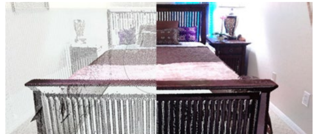
Figure 2. Comparison of high- and low-resolution point cloud (SCENE Workbook 2019)
