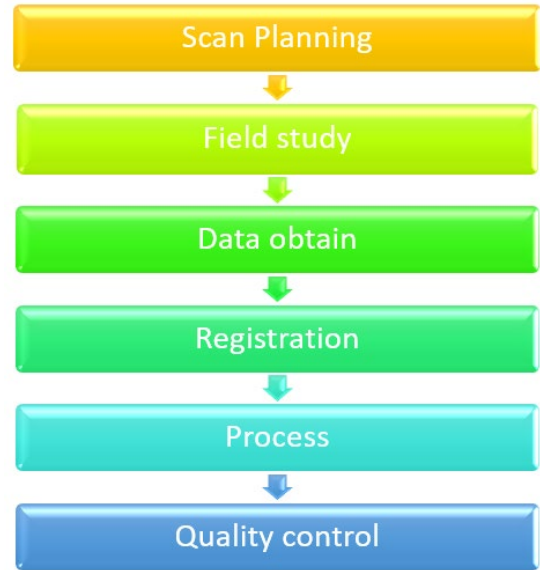
Figure 3. Process flow chart with TLS
