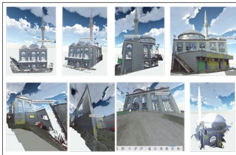
Figure 7. The view angles of 8 sessions after unnecessary points removal for manual registration.
