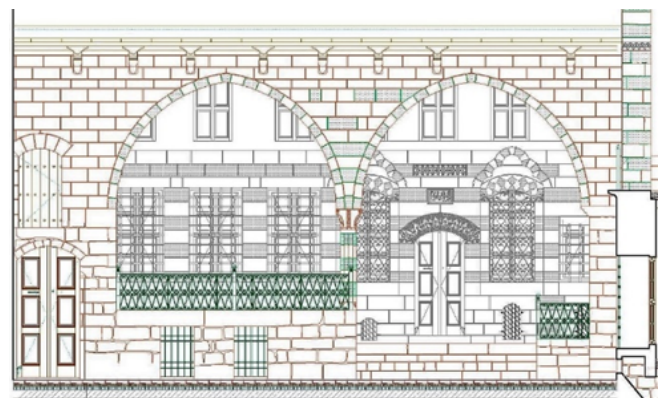
Figure 17. Analytical survey of the east façade of the building facing the courtyard
