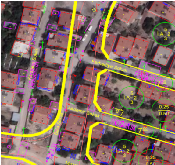
Figure 1. Example illegal structures on the zoning roads
