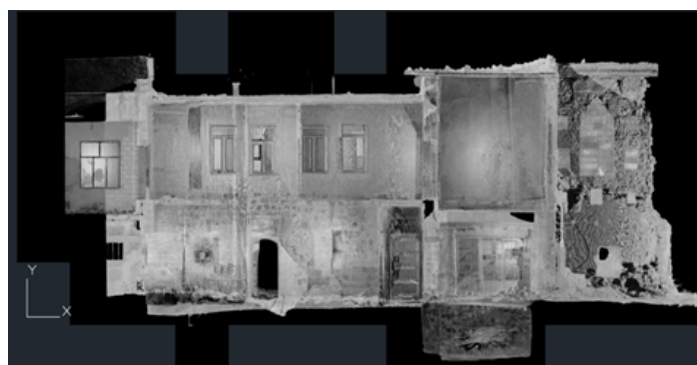
Figure 8. Orthophoto of the western façade
