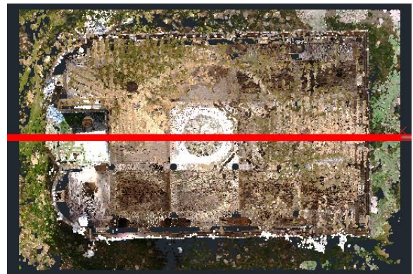
Figure 5. Section line over the 3D point cloud
