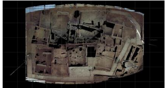
Figure 15. Plan of archaeological area without shelter from TLS data point cloud data in Scene software
