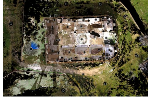
Figure 1. Stations used in scanning
