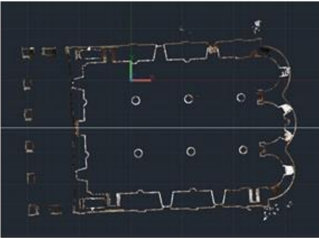
Figure 4. Point cloud slice plan section and drawing
