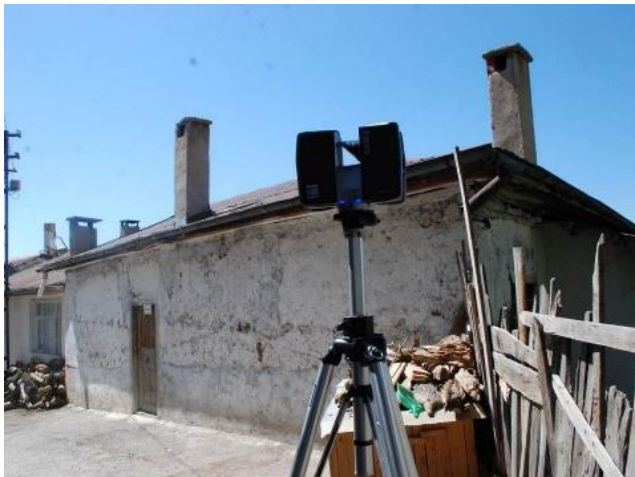
Figure 2. 3D Laser scanner of historical house
