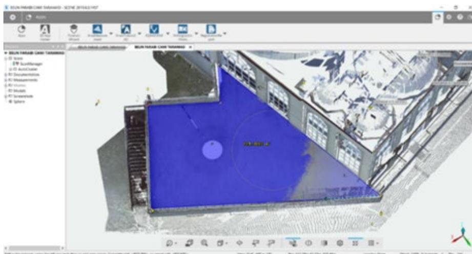
Figure 12. Calculation of terrace area in Scene 2019 software.
