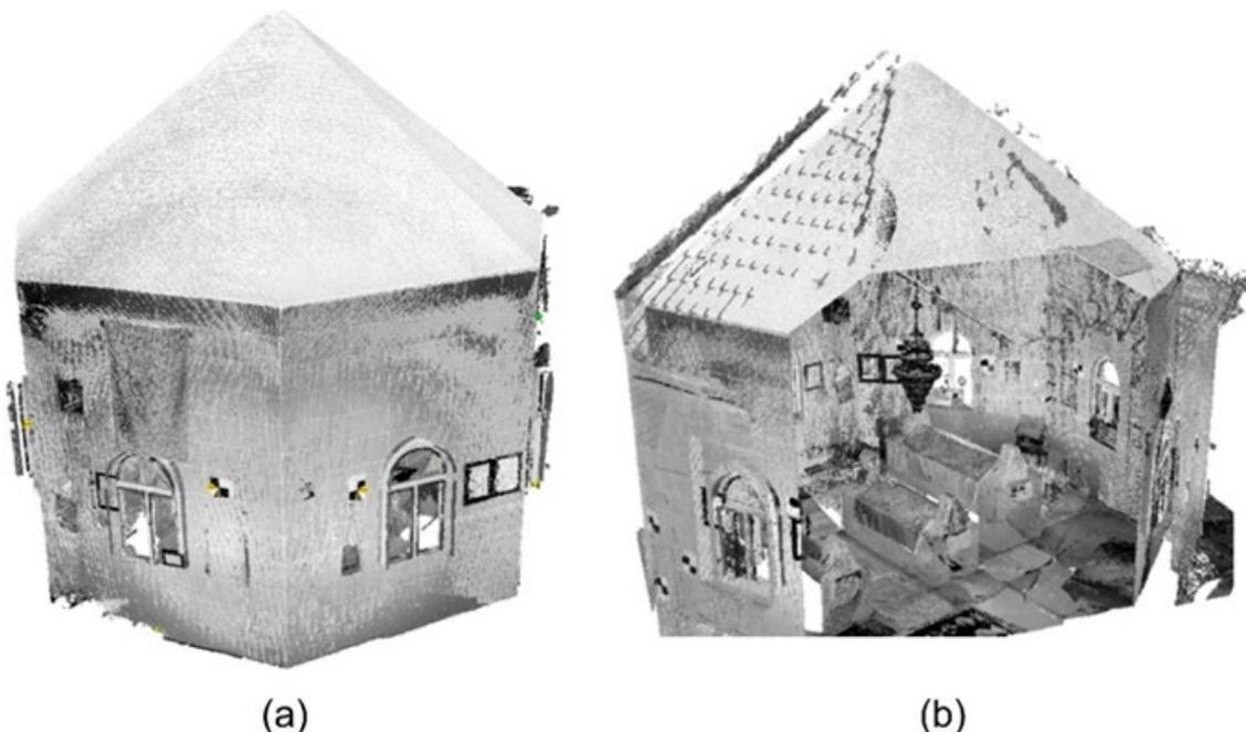
Figure 3. 3D point cloud of the tomb (outdoor) (a), indoor (b)
