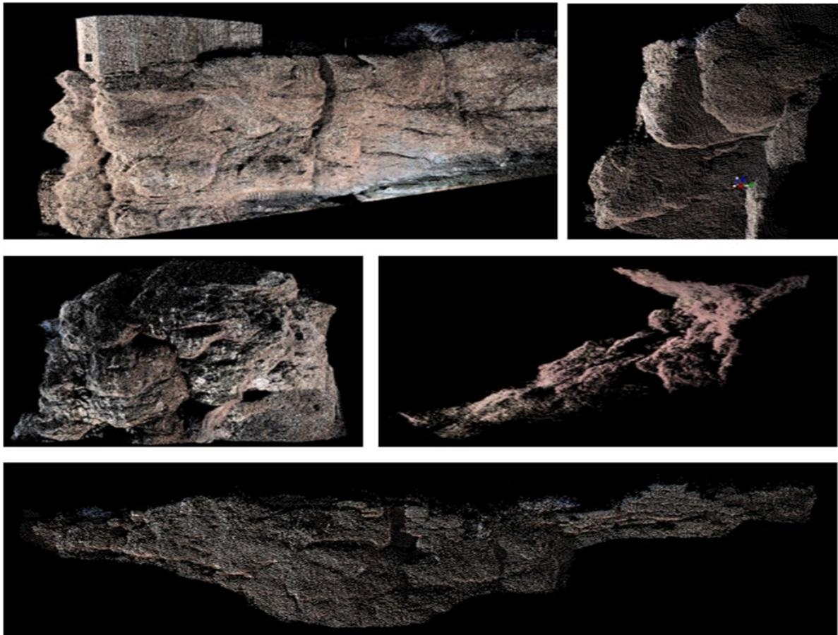
**Figure 4.** Examples of 3D point cloud images obtained by scanning the castle with a laser scanner (Mardin Metropolitan Municipality, 2023)
