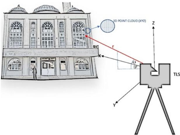
Figure 1. Data acquisition with terrestrial laser scanner
