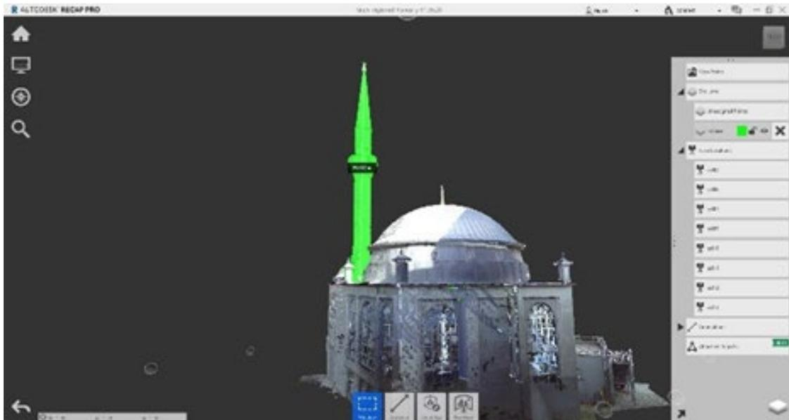
Figure 13. Minaret height measurement in Autodesk Recap 2020 software.
