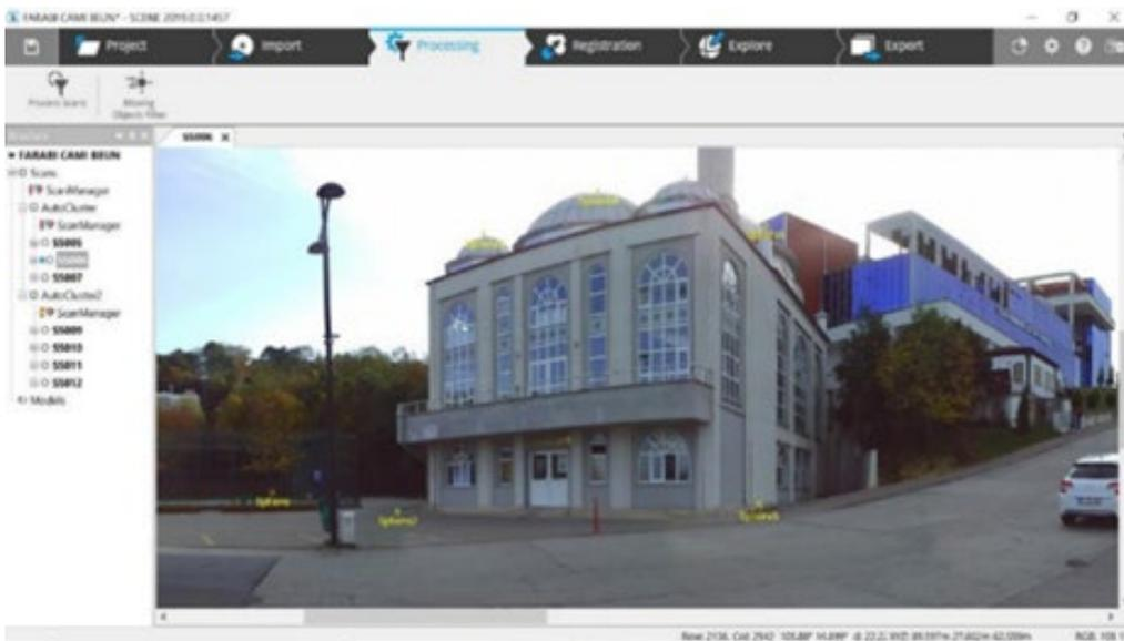
Figure 5. Automatic sphere selection phase of Scene 2019 software.
