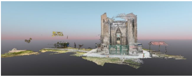
Figure 8. Unpurged version of the Ali Cafer Kumbet point cloud data (North facade).
