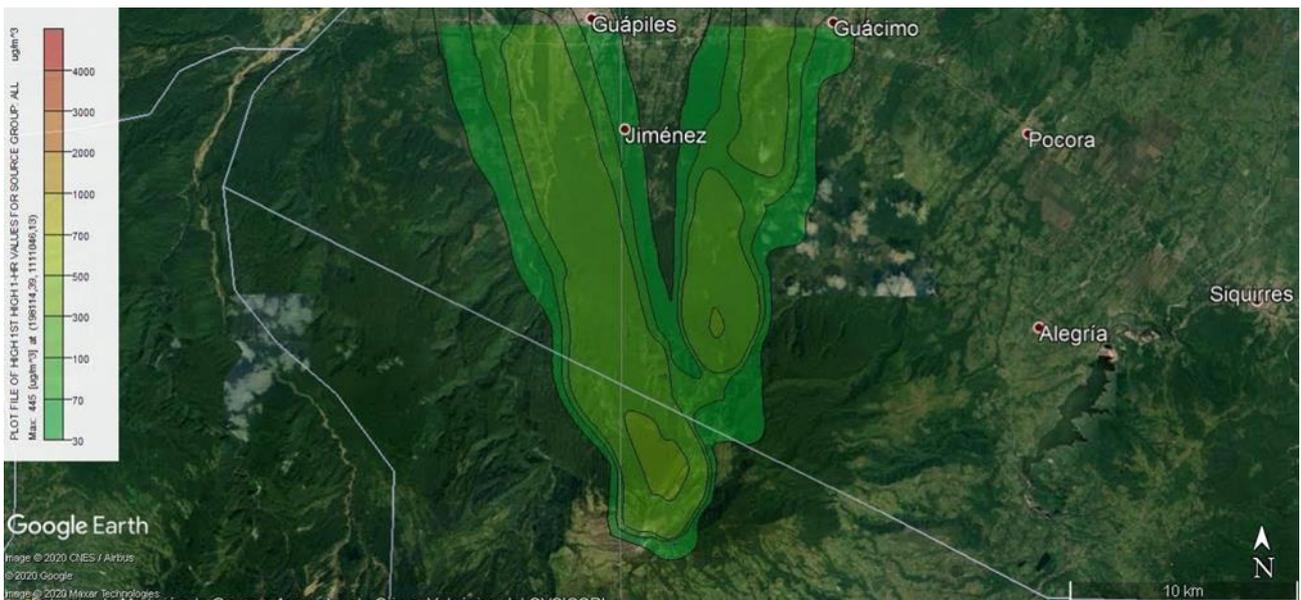
**Figure 88.** AERMOD plot of Turrialba Volcano emissions of SO<sub>2</sub> September 27<sup>th</sup>, 2022
