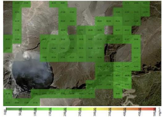
Figure 113 & 114. H<sub>2</sub>S & HF emissions tracked with Aki-01 in Sniffer Mapper software program
