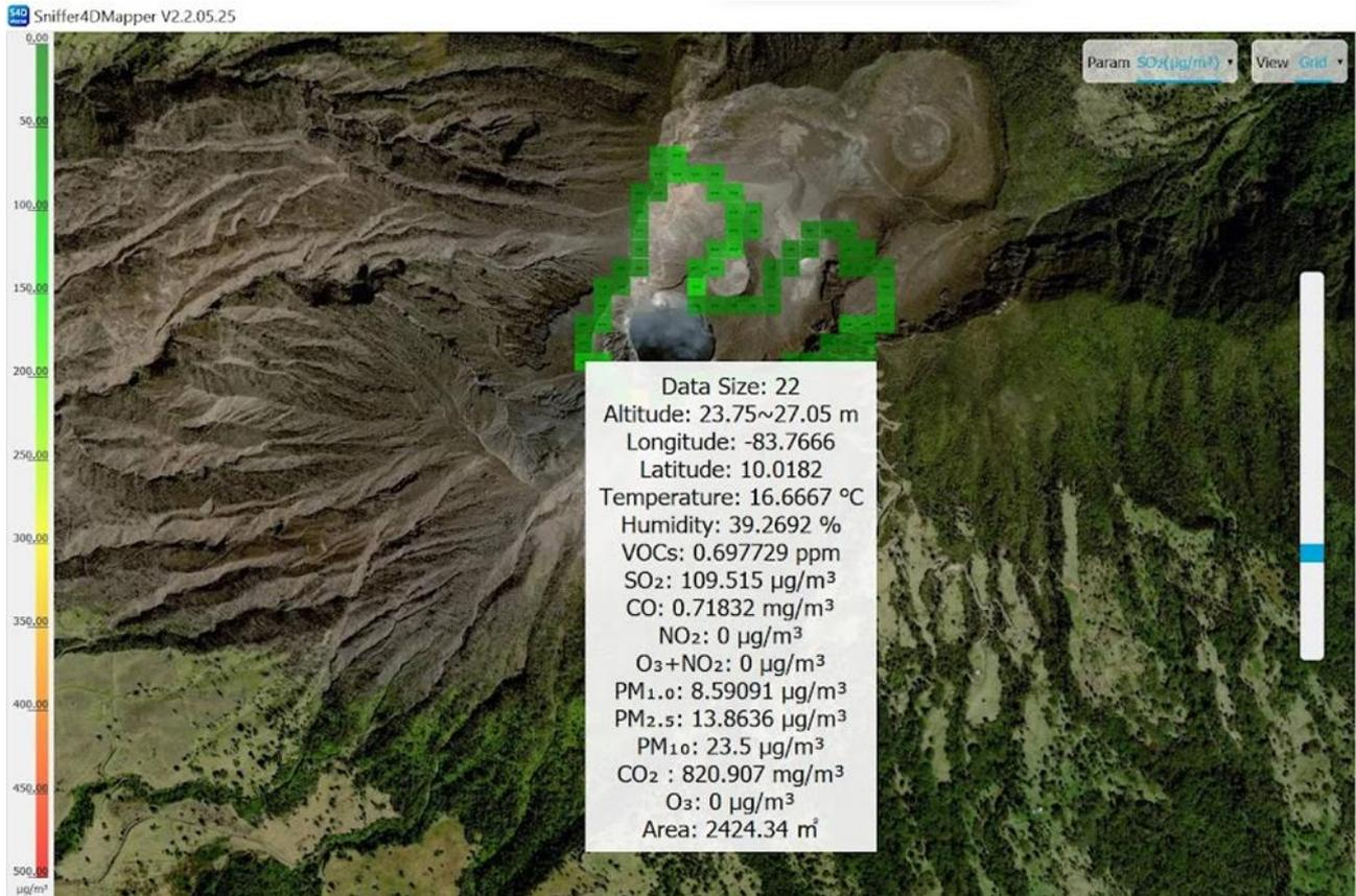
Figure 95. Sniffer4D measurements from the active west crater of the Turrialba Volcano
