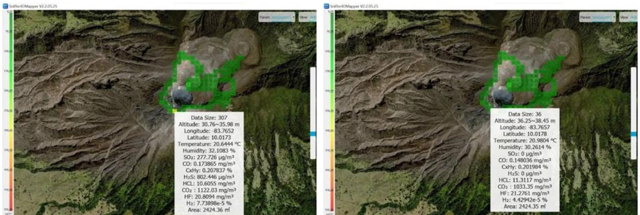
Figure 78 & 79. SnifferV & Sniffer4D emission tracking the active west crater of the Turrialba Volcano
