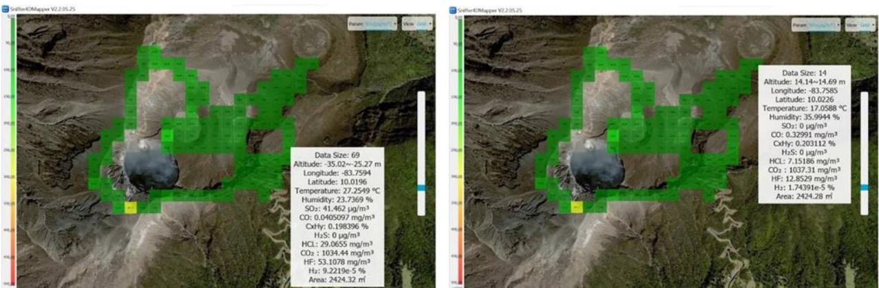
Figure 21 & 22. SnifferV & Sniffer4D ambient air monitoring at the east crater of the Turrialba Volcano
