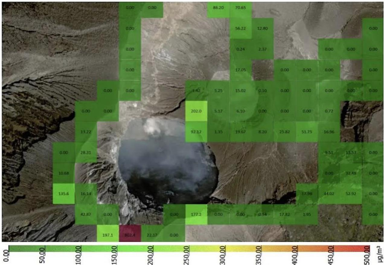
Figure 76. H<sub>2</sub>S emissions tracked in Sniffer Mapper software program
