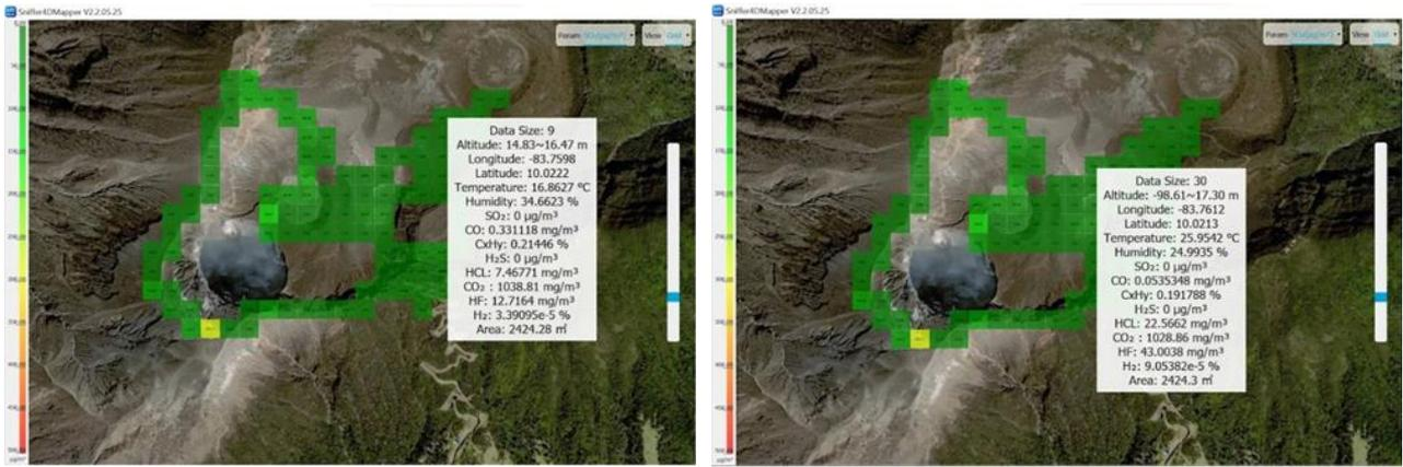
Figure 23 & 24. SnifferV & Sniffer4D ambient air monitoring at the east crater of the Turrialba Volcano
