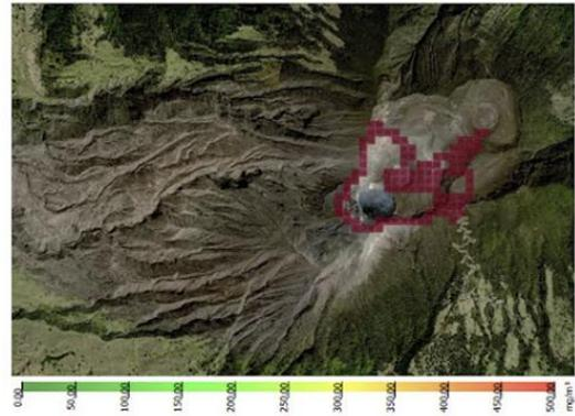
Figure 111 & 112. SO<sub>2</sub> CO<sub>2</sub> emissions tracked with Aki-01 in Sniffer Mapper software program
