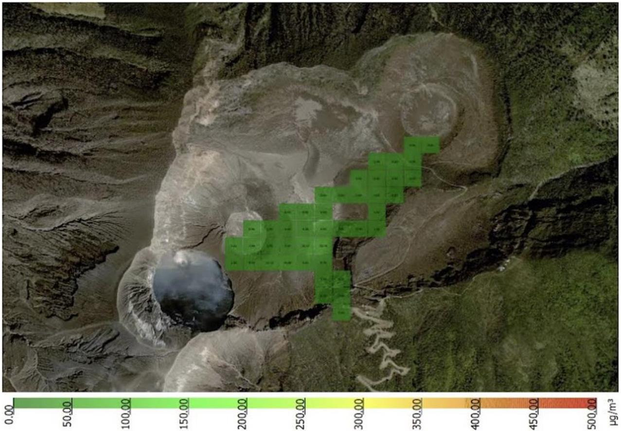
Figure 10. SO<sub>2</sub> Emissions tracked with Aki-01 in Sniffer Mapper software program
