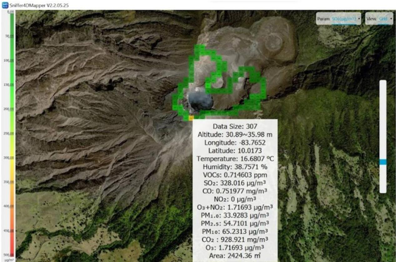
**Figure 87.** Sniffer4D measurements from the active west crater of the Turrialba Volcano
