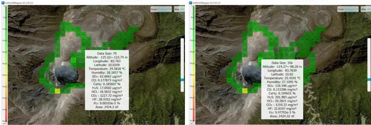
Figure 66 & 67. SnifferV & Sniffer4D emission tracking inside the central crater of the Turrialba Volcano
