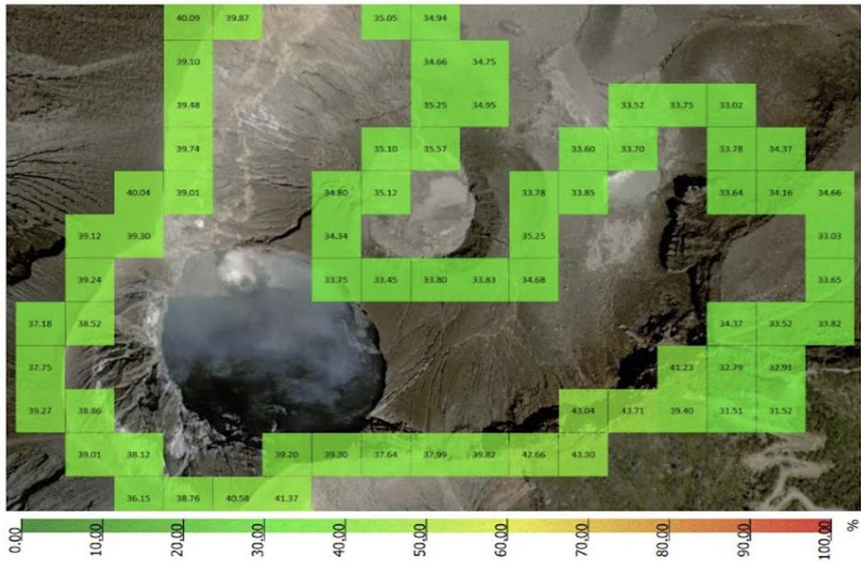
Figure 115. Humidity tracking on the Sniffer4D at the west & central craters of the Turrialba Volcano
