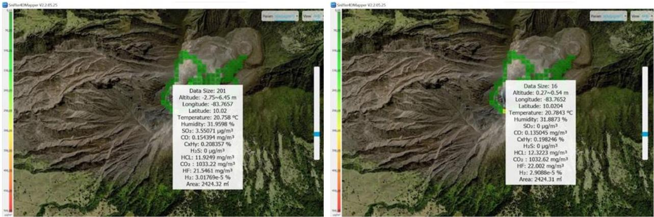
Figure 82 & 83. SnifferV & Sniffer4D emission tracking the active west crater of the Turrialba Volcano
