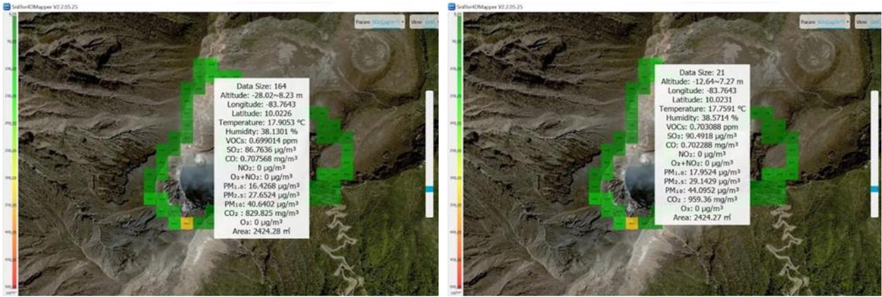
Figure 53 & 54. Sniffer4D measurements from the central crater of the Turrialba Volcano
