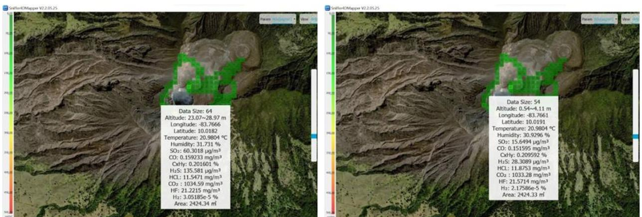
Figure 80 & 81. SnifferV & Sniffer4D emission tracking the active west crater of the Turrialba Volcano
