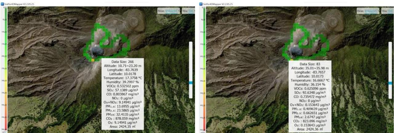
Figure 91 & 92. Sniffer4D measurements tracking from the active west crater of the Turrialba Volcano
