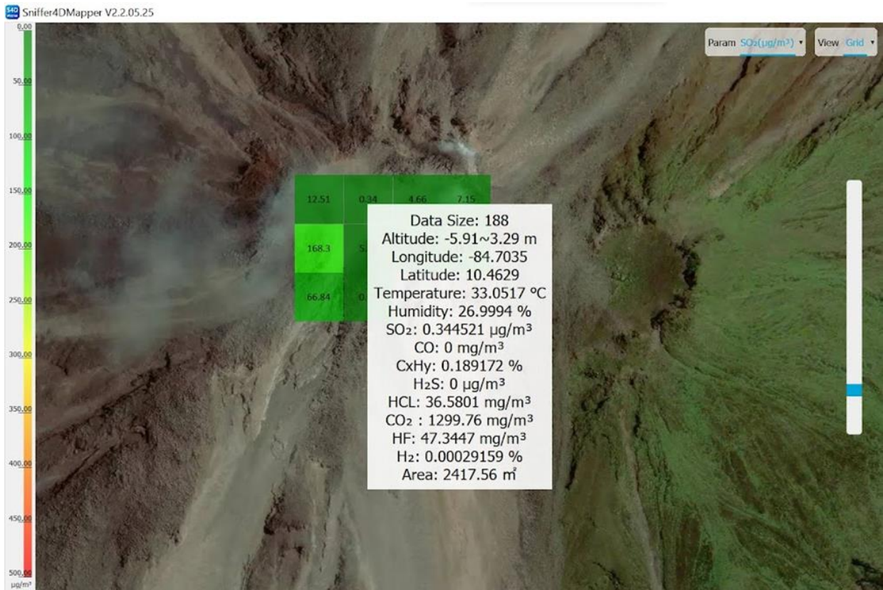
Figure 46. Measurements Taken from Degassing Fumarole of Active Crater C in Sniffer Mapper.
