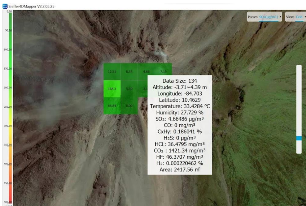
Figure 45. Measurements Taken from Degassing Fumarole of Active Crater C in Sniffer Mapper.
