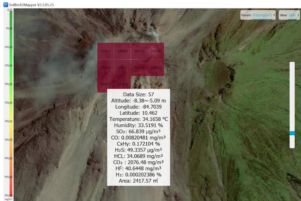
Figure 50. SnifferV Measurement Taken from Area of Most Significant Degassing.
