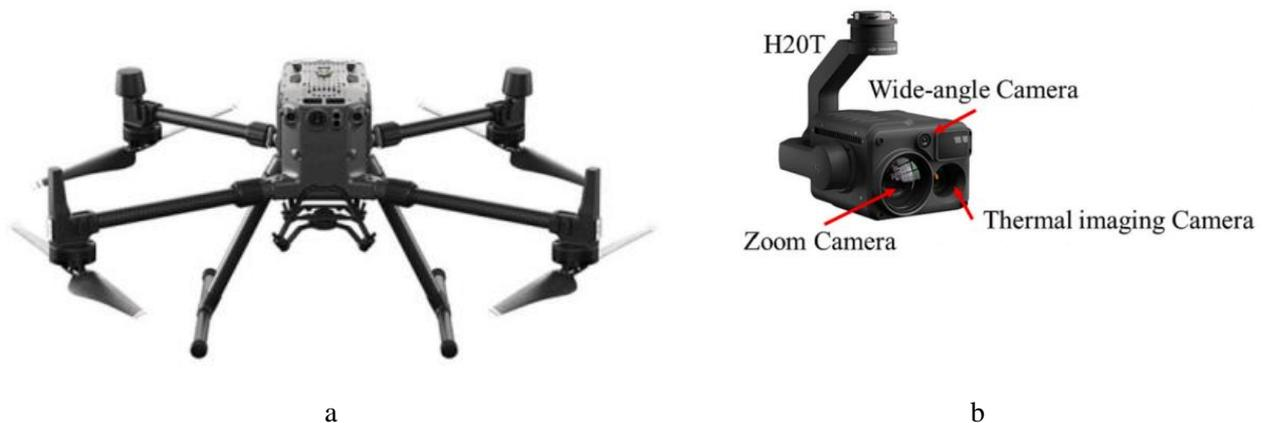
**Figure 12.** Research objects and equipment. (a: M300 RTK UAV, b: H20T camera.)
