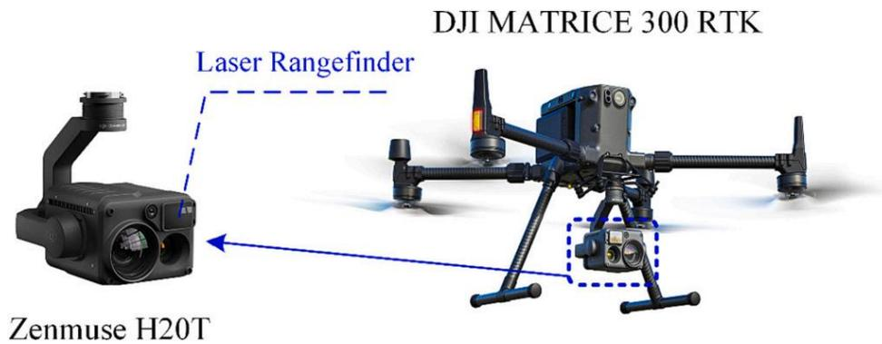
**Figure 11.** Components of UAV system.
