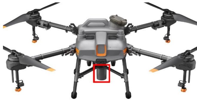
Figure 22. An agricultural UAV with a radar sensor [47].
