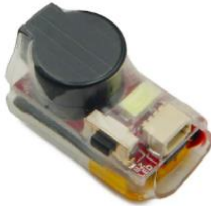
Figure 11. Missing UAV locator sensor (buzzer) [17].
