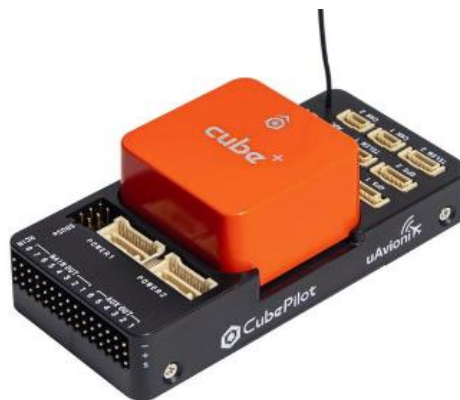
Figure 7. UAV flight control system (it has 3 IMUs) [12].
