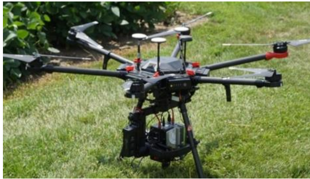
Figure 5. UAV system with multiple GNSS receivers [9].
