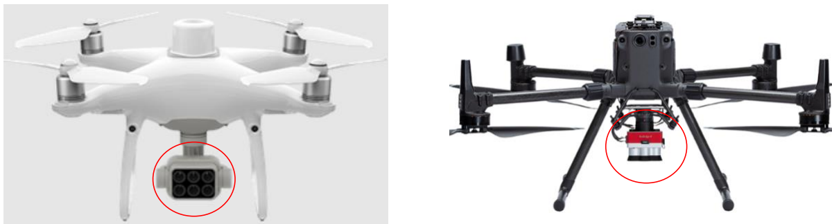
Figure 16. UAV on-board (A) and post-integrated (B) multispectral cameras [33, 34].
