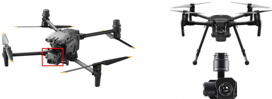
Figure 18. Thermal cameras on the UAV (A) and subsequently integrated (B) [37, 38].
