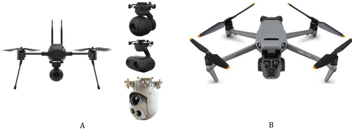
Figure 1. UAV models with different types of sensors. A: UAV model with replaceable electro-optical sensors, B: UAV model with integrated electro-optical sensor [5, 6].
