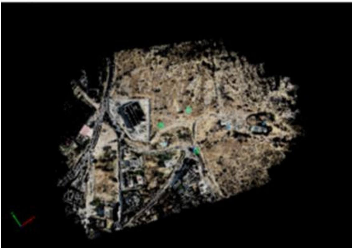
Figure 5. Presentation of ground control points in the working area through the software program
