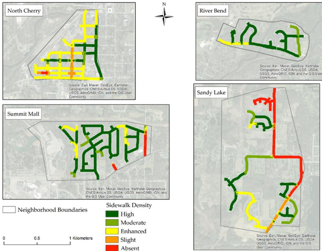
Figure 5. The spatial distribution of sidewalks. (a) high, denoting two-sided sidewalks the whole way; (b) denoting a street segment with two-sided and one-sided sidewalks; c) enhanced, denoting three variations in a street segment: two sides, one side, and no sidewalks; (d) slight, denoting a segment with one side and no sidewalks; and (e) absent, denoting no sidewalks in the entire segment [8]
