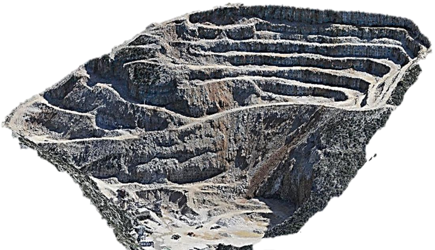
Figure 4. Mine excavation site point cloud
