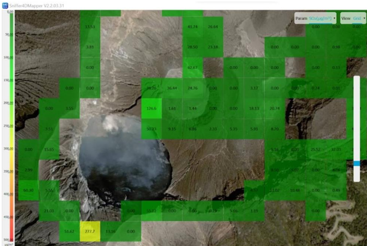
Figure 25. Sniffer4D Data on SO 2 Showcased on the Sniffer Mapper software program
