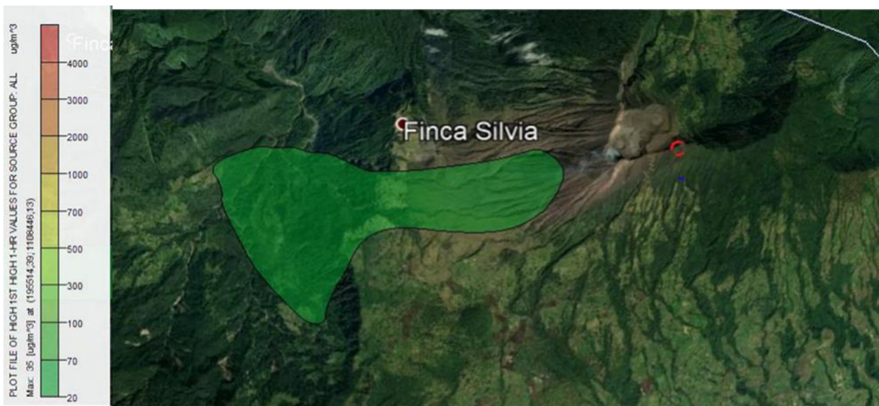
Figure 18. AERMOD Plot from April 8 th , 2022 the day of investigation with the Sniffer4D the SO 2 emission that day was around (151 +/- 142) ton/day which was supported by the Sniffer4D data from the crater
