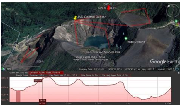
Figure 8 & 9. Autel Lite + (Red) Operational Flight Missions Altitude and Terrain Check Diego Crater Irazú Volcano
