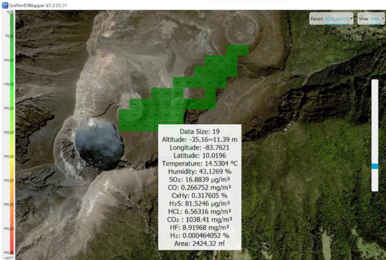
Figure 24. Sniffer4D Data on SO 2 Showcased on the Sniffer Mapper software program
